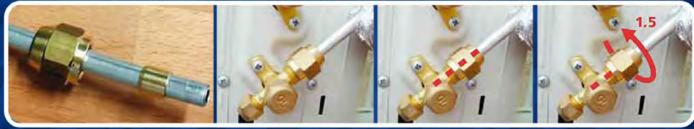
Insert tube, cut and deburred, into the nut; then insert sleeve.  Hand tighten nut to the joint.  Mark the starting point and rotate 1½ turns with standard wrench
